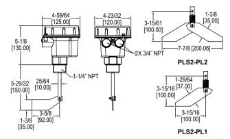
The Series PLS2 Paddle Level Switch is an electromechanical level switch designed for level monitoring of bulk materials. The rotating measuring vane is driven by a brushless synchronous motor at one revolution per minute and as product builds up, the paddle rotation is impeded and the resulting motor torque activates the output switch and stops the motor. The PLS2 is designed with the industry standard 1-1/4" male NPT connection and unit can be side or top mounted.
